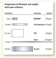
And unlike some materials, the multipurpose substrate is resistant to breakage, can be exposed to any kind of weather, and provides sound and vibration dampening. Dibond's rigid panels often require little or no substructure support, saving you material costs.
