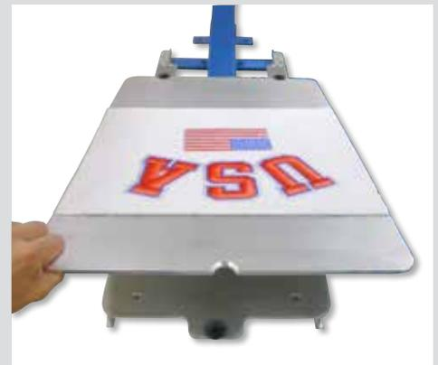
**Link Pallet unlocked and ready to move to another press or printer**
